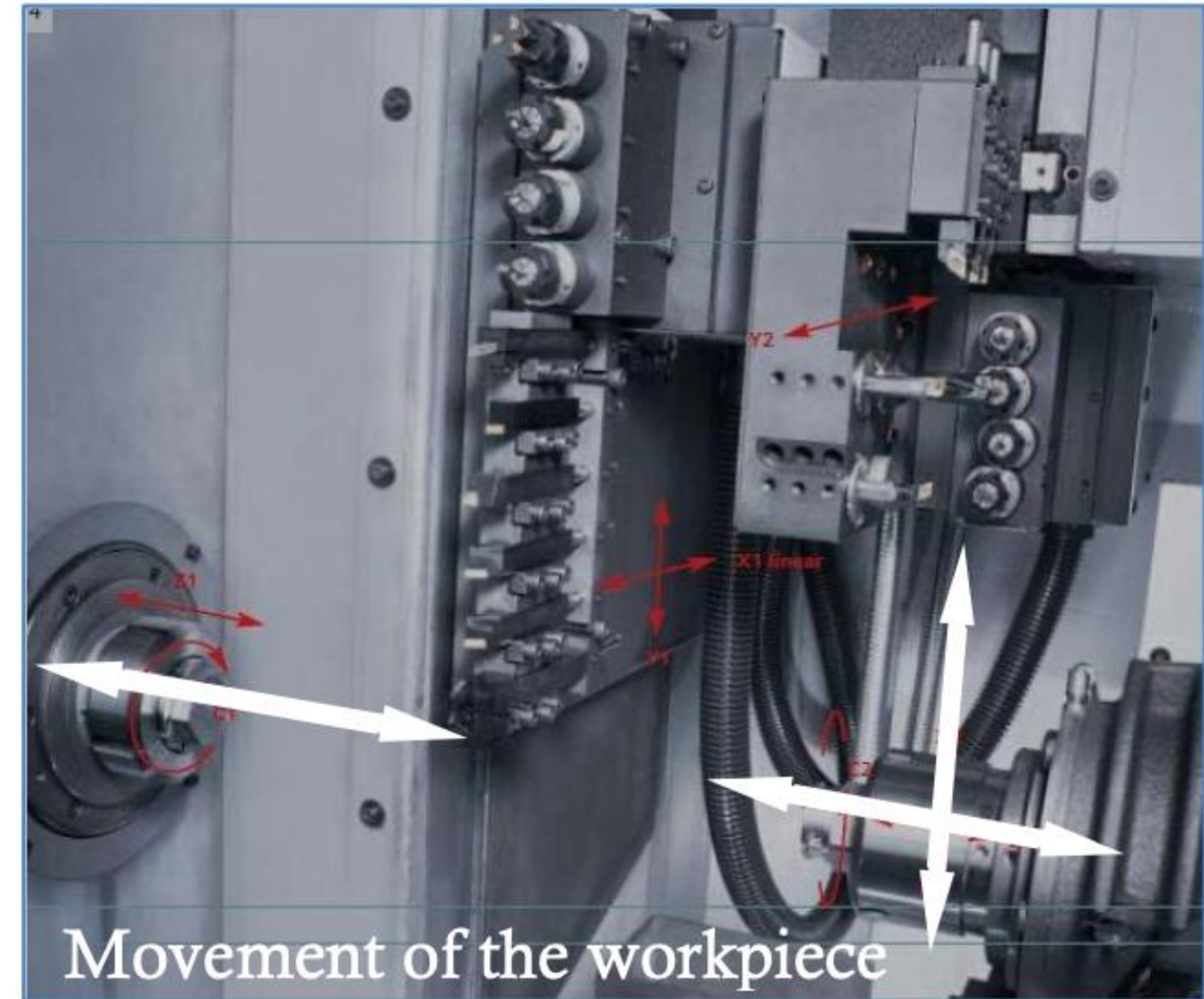
Fig. 29. Lathe with real movement of the Z-axis and of the X-axis on the workpiece
