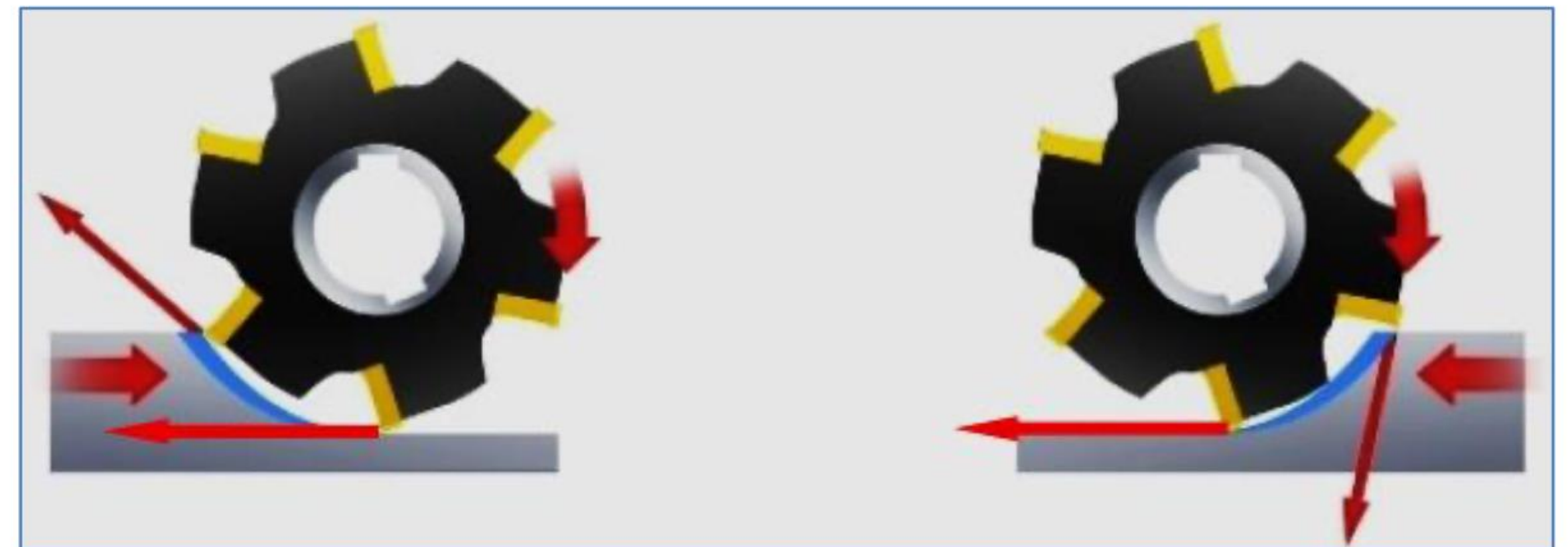
Fig. 153. Discordant cutting direction (left) and concordant cutting direction (right)
