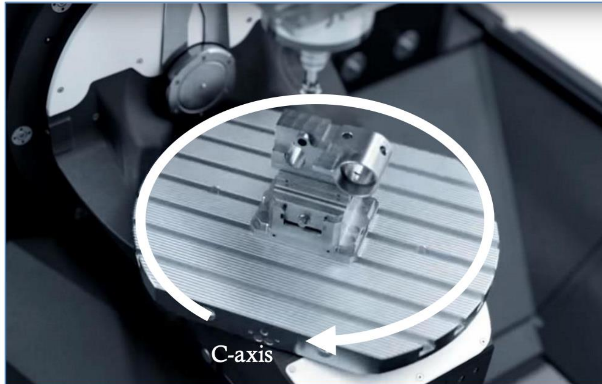
Fig. 130. C-axis in a machining center
