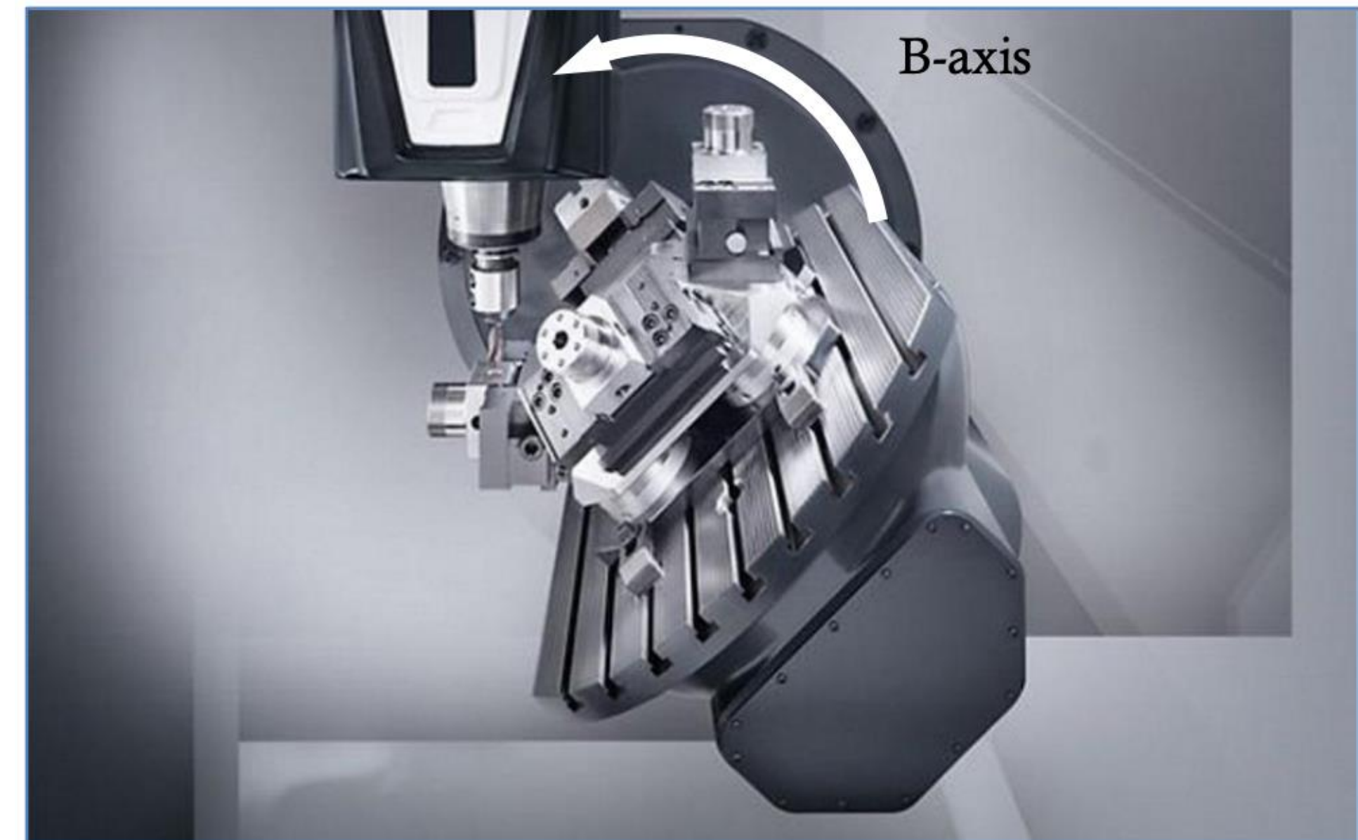
Fig. 131. B-axis in a machining center
