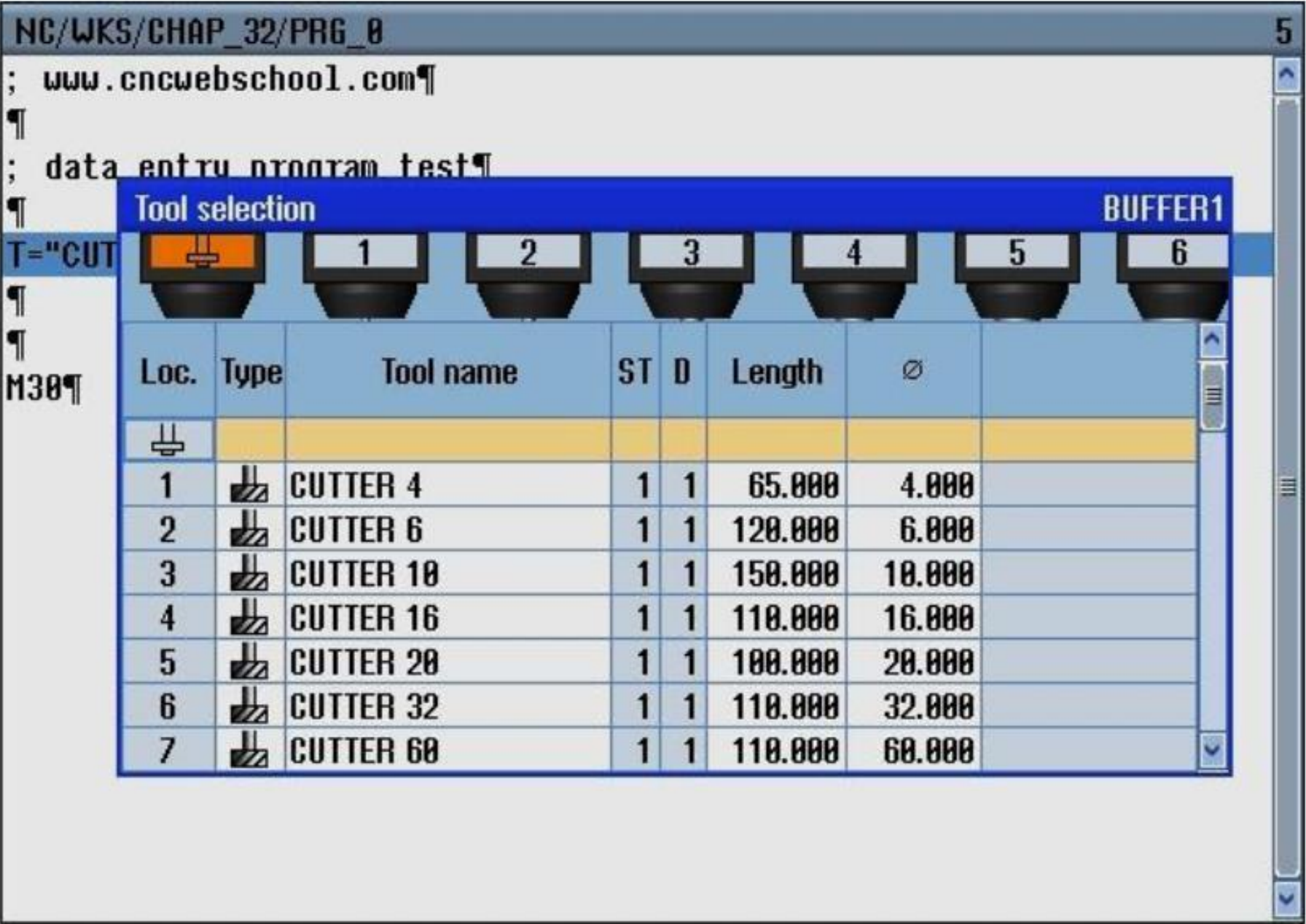
Fig. 139. Page for the selection of the tools directly from the magazine
