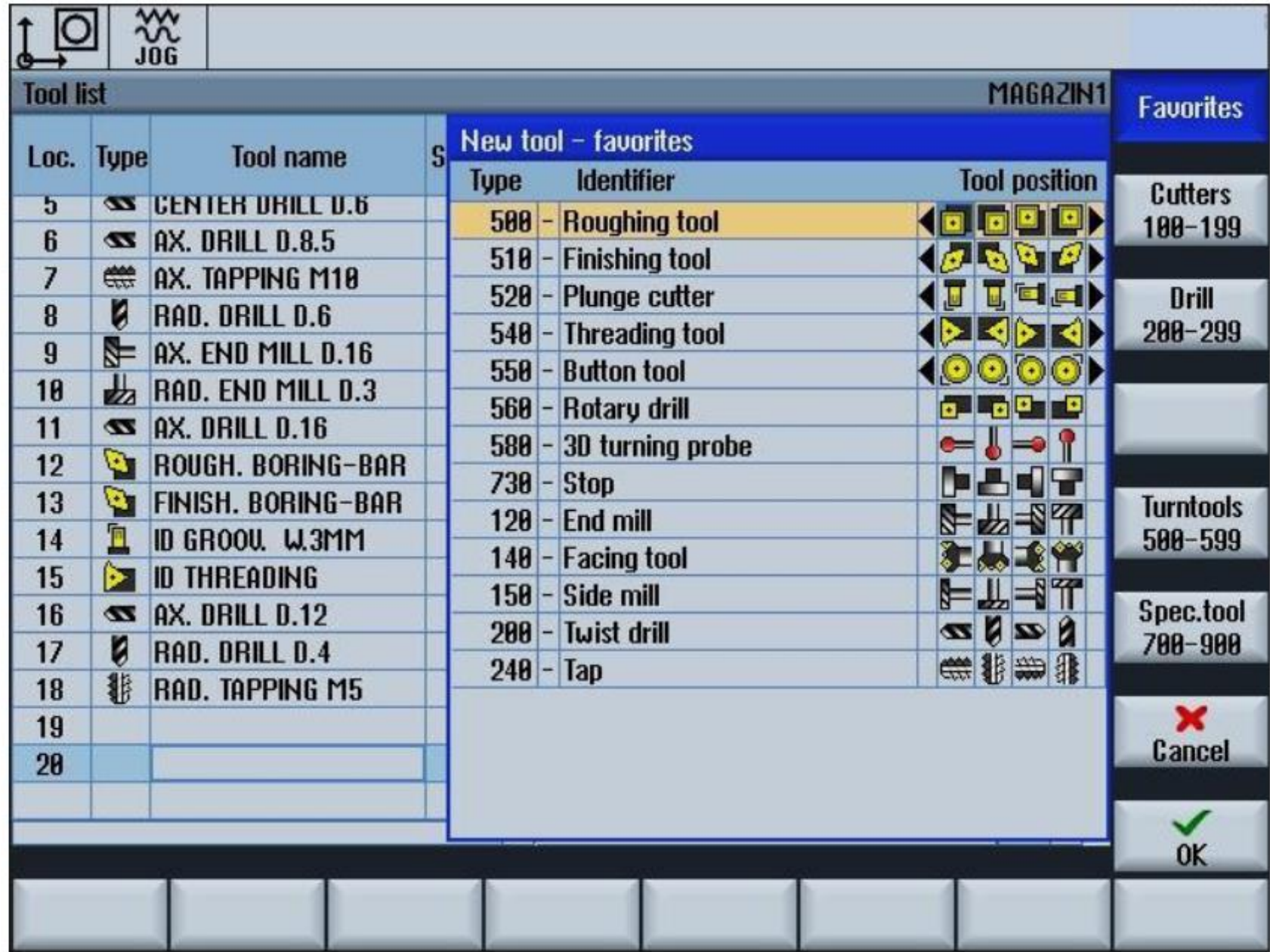
Fig. 67. Selection of the type of new tool to be created and position of the cutting edge
