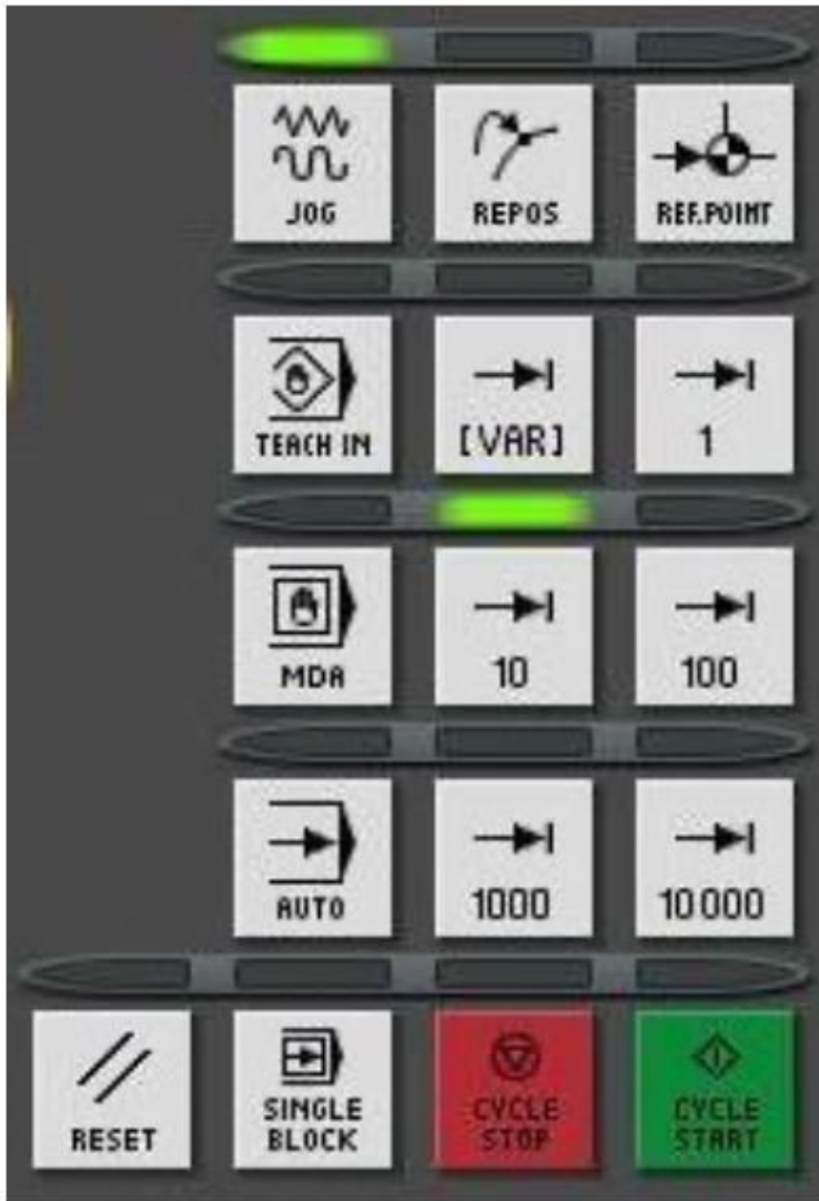
Fig. 57. Buttons for the selection of the manual feed by incrementation
