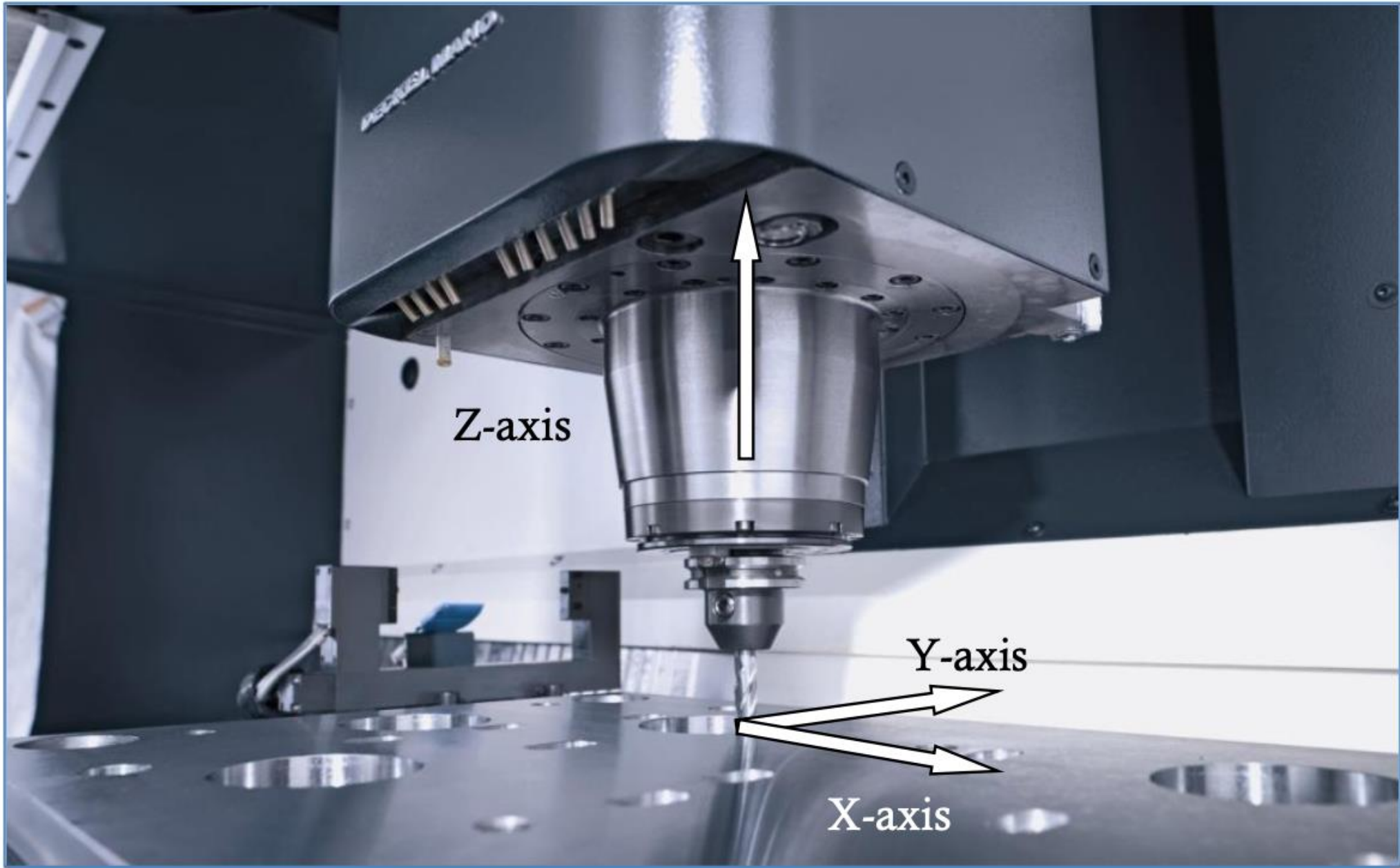
Fig. 2.1 Milling machine with 3 axes
