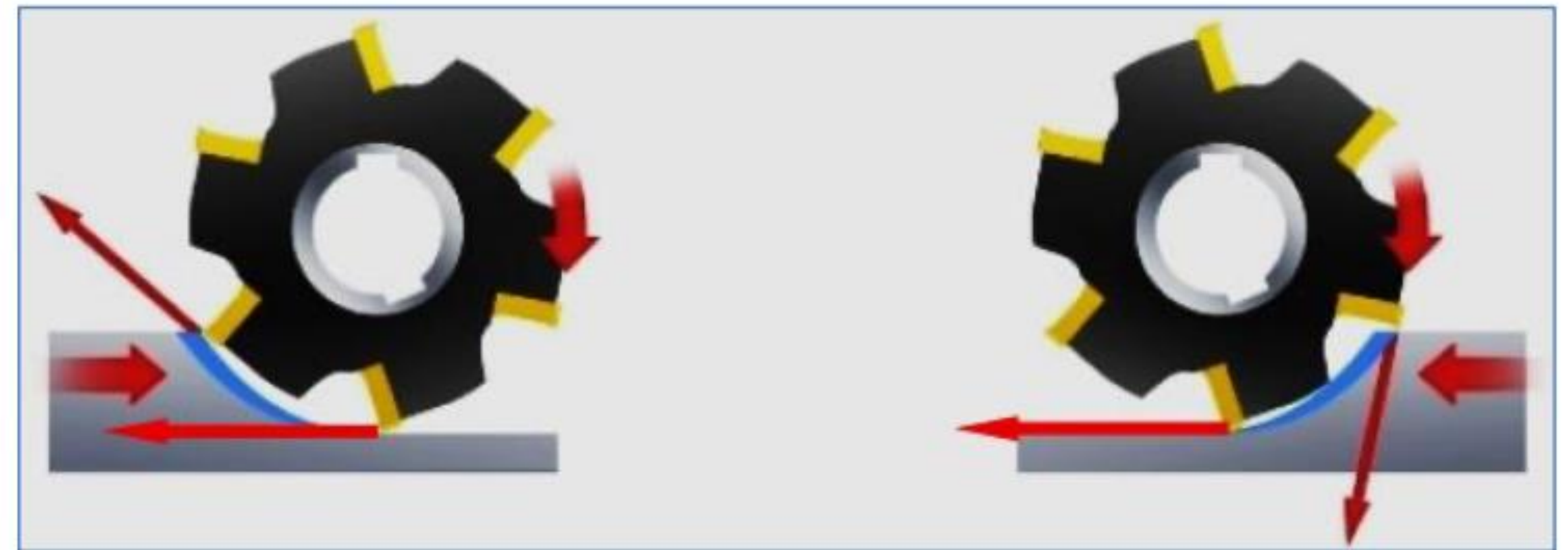
Fig. 233. Discordant cutting direction (left) and concordant cutting direction (right)
