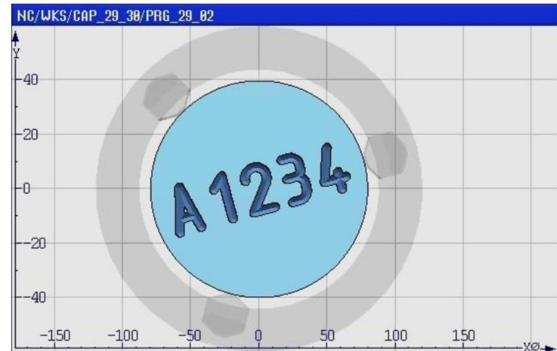
Fig. 190. Use of the engraving cycle to write on the front face of the workpiece
