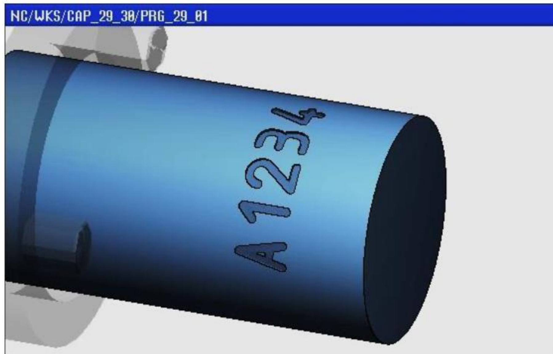
Fig. 189. Use of the engraving cycle to write on the circumference
