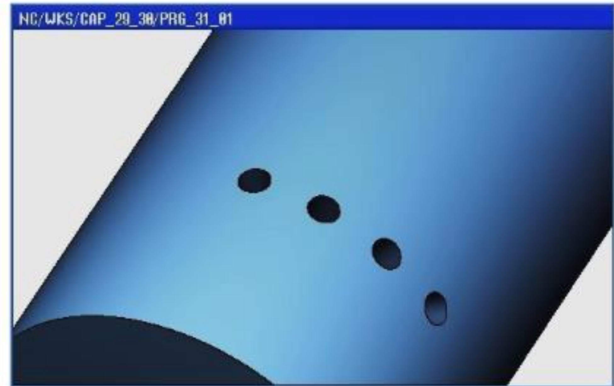
Fig. 204. Execution of a series of holes with constant lead, but not distributed over 360°
