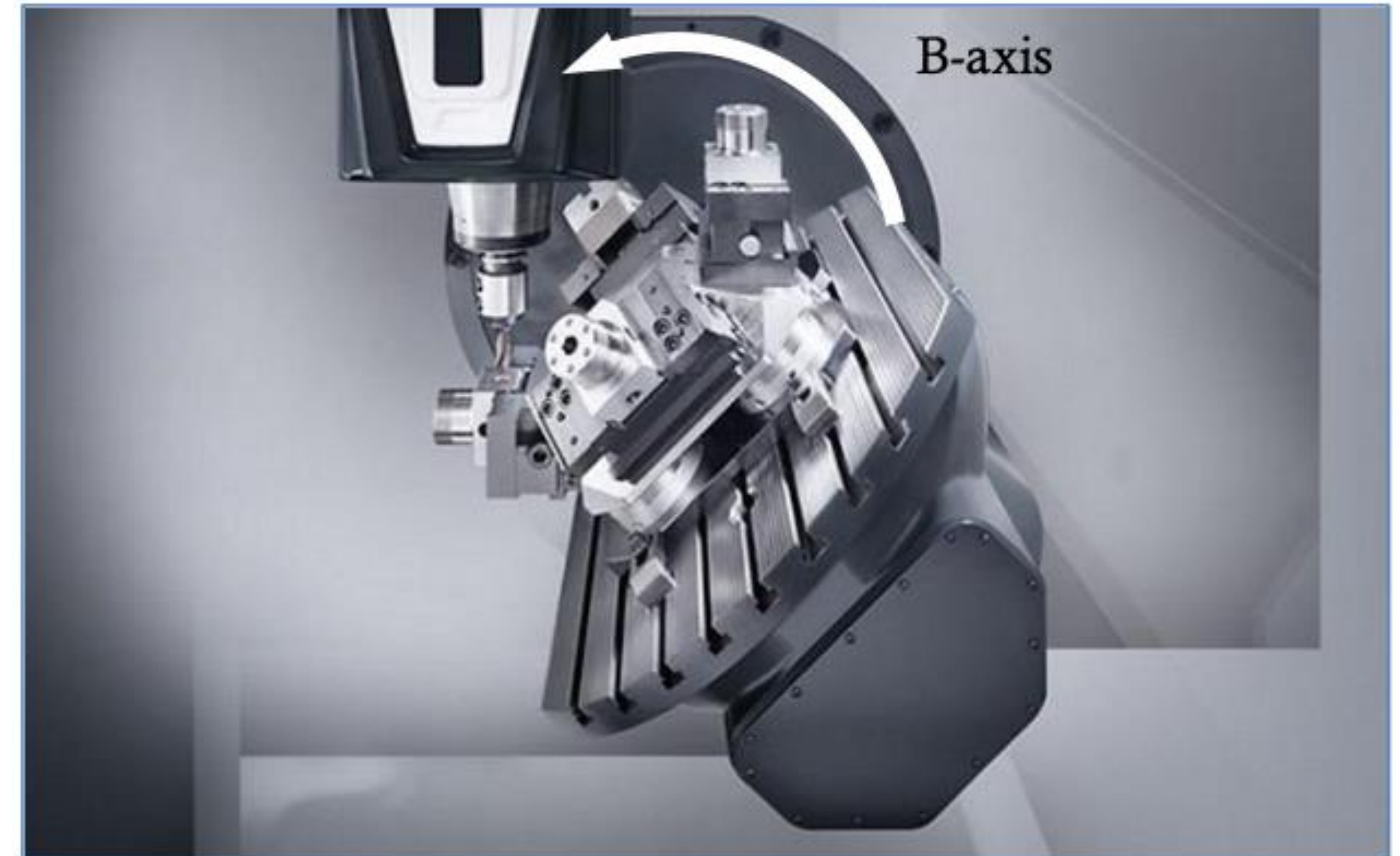
Fig. 211. B-axis in a machining center
